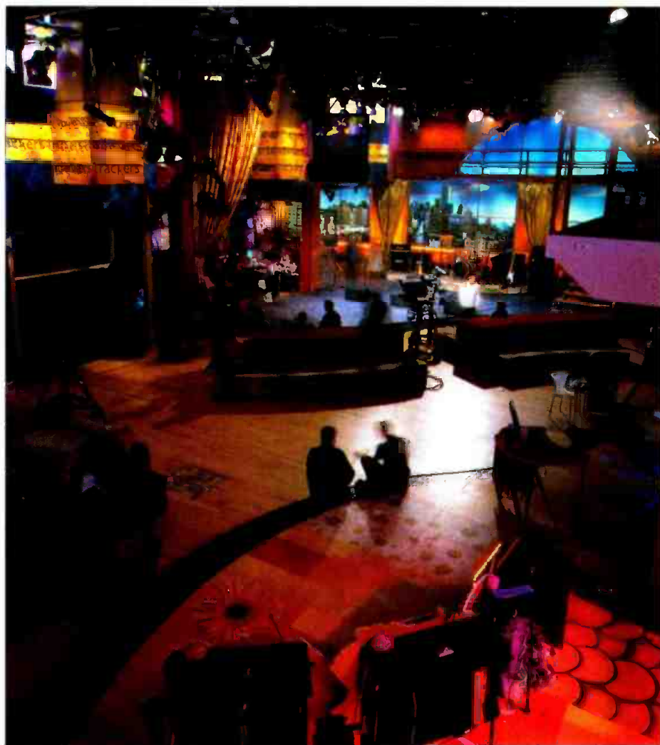
The Trackers studio located over 800 feet from the core production facility utilizes a Telecast Fiber Optic transmission system to provide interconnectivity to the central equipment room.
