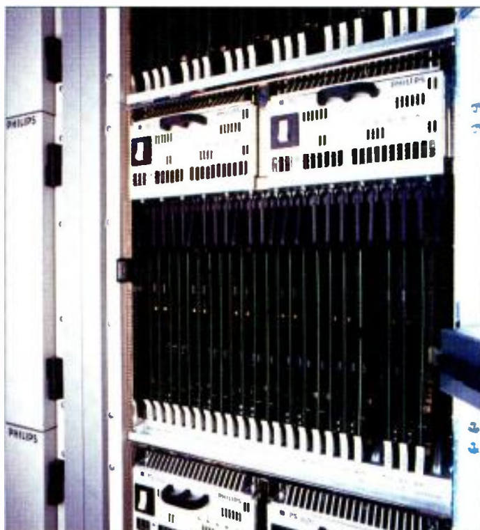
Large routing systems can take considerable rack space. Be sure to plan for sufficient rack space and cooling for the system chosen.
