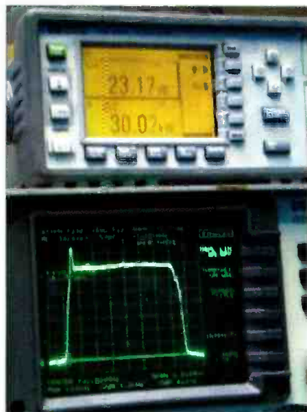
Figure 1. Spectrum analyzer and power meter showing the results of 8VSB modulation through a TH770/TH18770 system at 30kW (avg.) output power.
